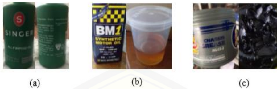
a) Minyak singer (ISO VG 15), b) Oli (SAE 10W-40), c) Grease (NLGI 3)
