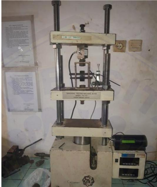
Gambar 3.6 Mesin uji tarik standart *universal machine testing* ESSOM TM 113.
