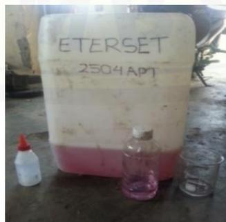
Gambar 2.15 Resin *unsaturated polyester Eterset 2504*.
