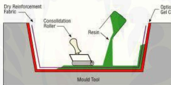
Gambar 2.4 Metode *hand lay up* (Sumber: Setyanto, 2012).
