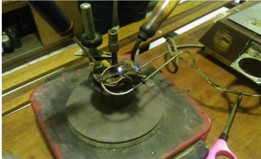
Gambar B6 Alat Uji Flash Point
