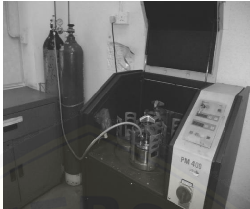
Gambar 2.4 Planetary BallMill Sizer (sumber: M Ramezani, 2012)
