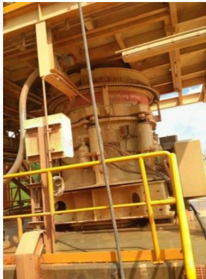
Gambar 2.1 Cone crusher Metso Nordberg HP500 (Sumber: PT. BSI, 2019)
