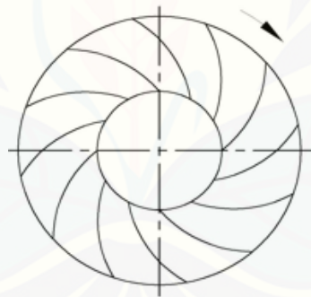
Gambar 2.2 Bilah type Backward Curved Blade (Onny, 2017).
