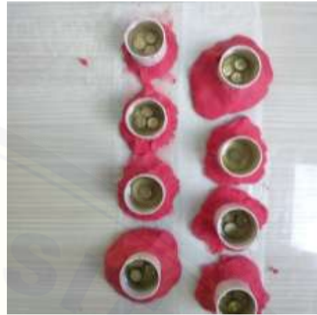
Mounting uji mikro
