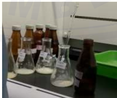
Gambar 3.13 Penambahan 2-3 tetes larutan campuran \text{HClO}_4 : \text{HNO}_3 (2:1)
