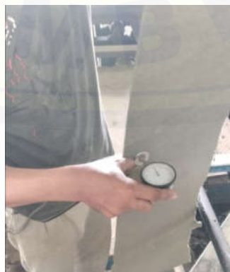
Lampiran 10: Proses pengukuran ketebalan wet sheet
