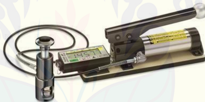
Gambar 3. 2 Pull of Test Adhesion Tester (Elcometer,2019)
