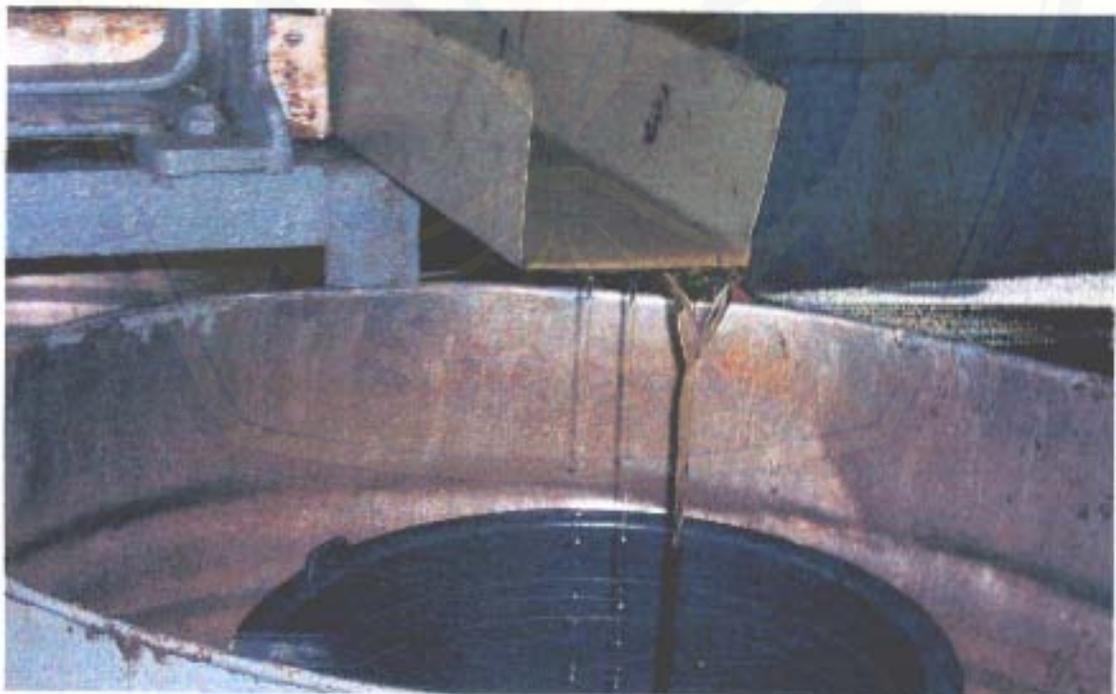
Gambar 18. Hasil Minyak Proses *Filter Press*
