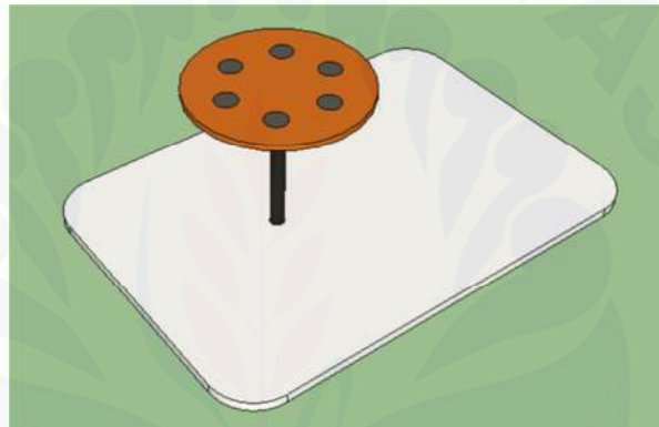
Gambar 3.5 Perancangan Rotor Motor BLDC ( Brushless Direct Current ) Fluks Aksial
