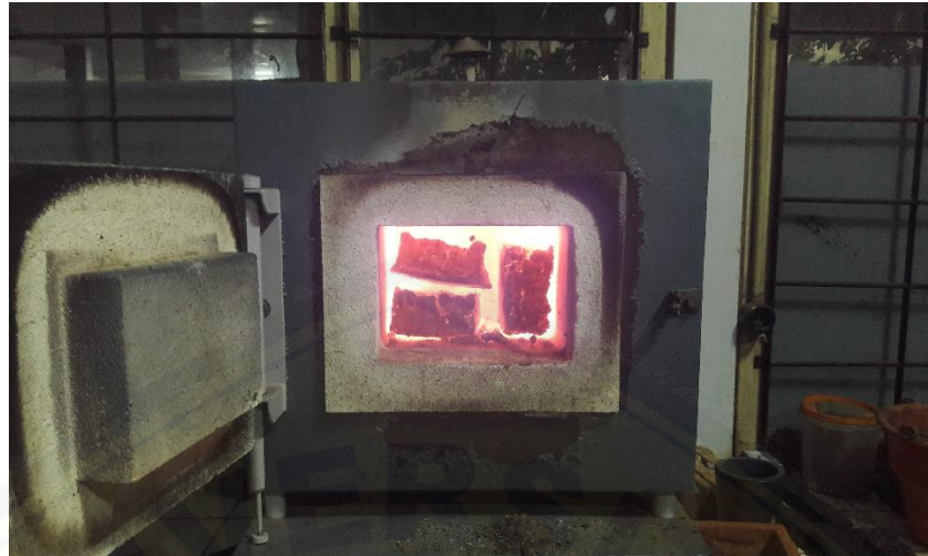
Gambar 3.3 Mesin Furnace Kenaikan Suhu Furnace
