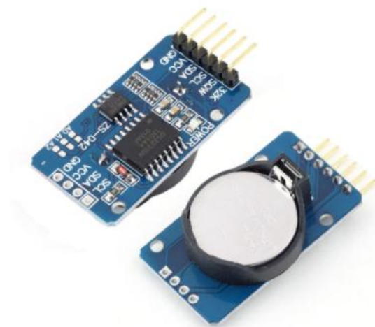
Gambar 2.3 Modul RTC ( Realtime clock ) DS3231
