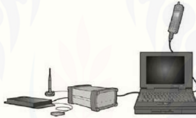
Gambar 2.5 Konfigurasi drive test MS-receiver
