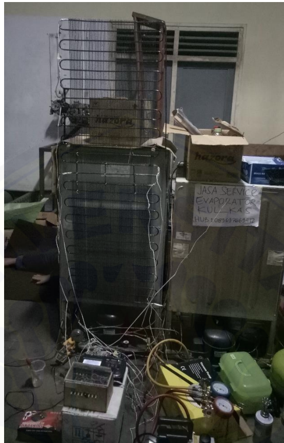
Gambar G.13 Proses perakitan separation condenser
