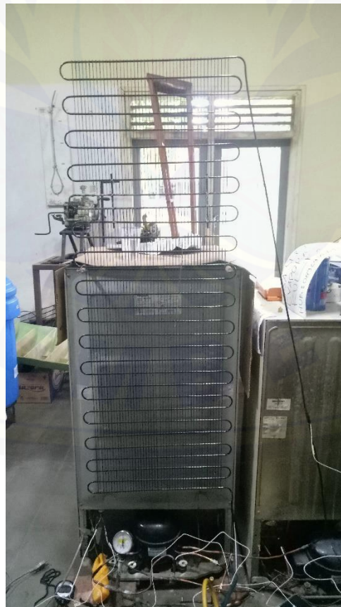
Gambar G.12 Proses perakitan baseline condenser
