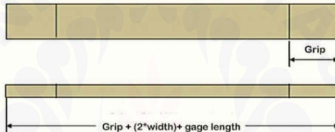
**Gambar 2.3 Sampel Uji Tarik ASTM D-3039 (ASTM, 1990)**
