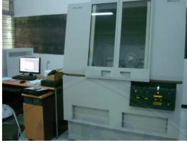
Gambar 3.4 Alat uji XRD merk PanAnalytical , Type: E'xpert Pro
