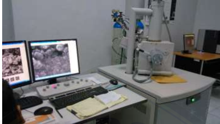
Gambar 3.3 Alat uji NDT SEM FEI merk Impact S50
