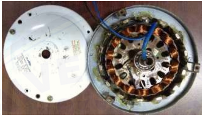
Gambar 1. Hasil Generator rewinding
