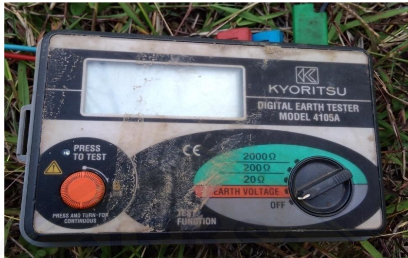
Alat Pengukuran tahanan grounding ( Earth Tester )
