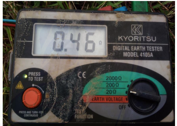
Alat Pengukuran tahanan grounding ( Earth Tester )
