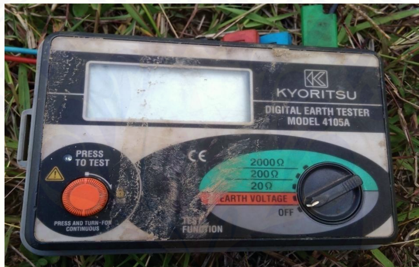
Gambar 3.2 Earth Tester Kyoritsu Model 4105A
