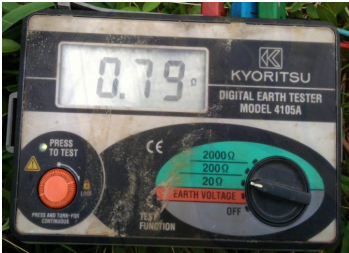
Alat Pengukuran tahanan grounding ( Earth Tester )
