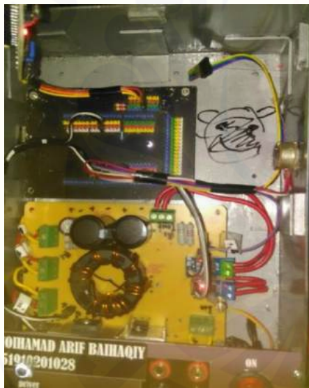
B3. Gambar SEPIC Converter
