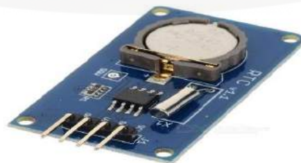
Gambar 2.10 Modul Real Time Clock ( RTC ) DS1307
