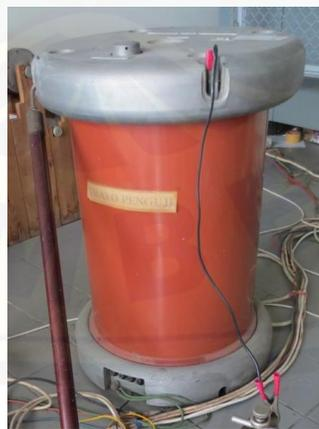
Gambar 3.2 Transformator *Step-up*
