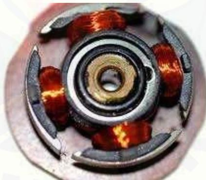
Gambar 2.10 Gambar Stator Pada Motor *Brushless* DC (Dirjis, 2012)
