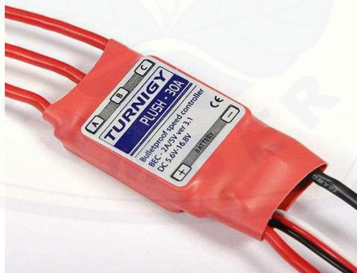
Gambar 2.12 *ESC (Electronic Speed Controller)* (solehudin, 2013)
