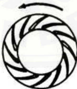
Gambar 2.2 Blower sentrifugal tipe Backward Curved Blade (Onny, 2017).
