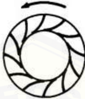
Gambar 2.1 Blower sentrifugal tipe Forward Curved Blade (Onny, 2017).
