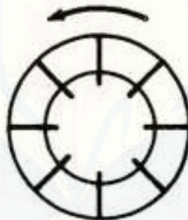
Gambar 2.3 Blower sentrifugal tipe Straight Curved Blade (Onny, 2017).
