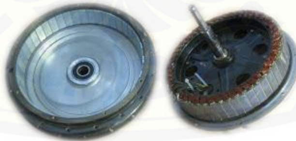
Gambar 2.1 Rotor dan stator motor Brushless Direct Current
