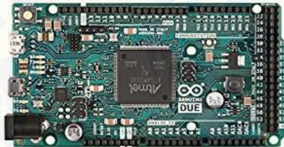
Gambar 2.6 Modul ARM Cortex-M3 AT91SAM3X8EA
