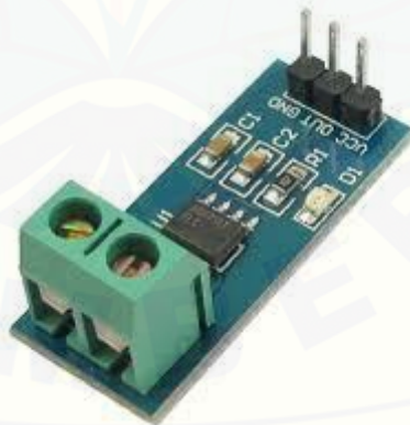
Gambar 2.7 Sensor Arus ACS712
