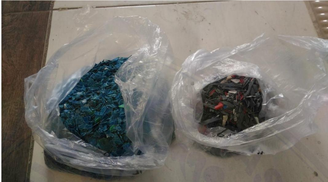
Gambar B.1 Plastik *low density polyethylene* (LDPE) dan *polystyrene* (PS)
