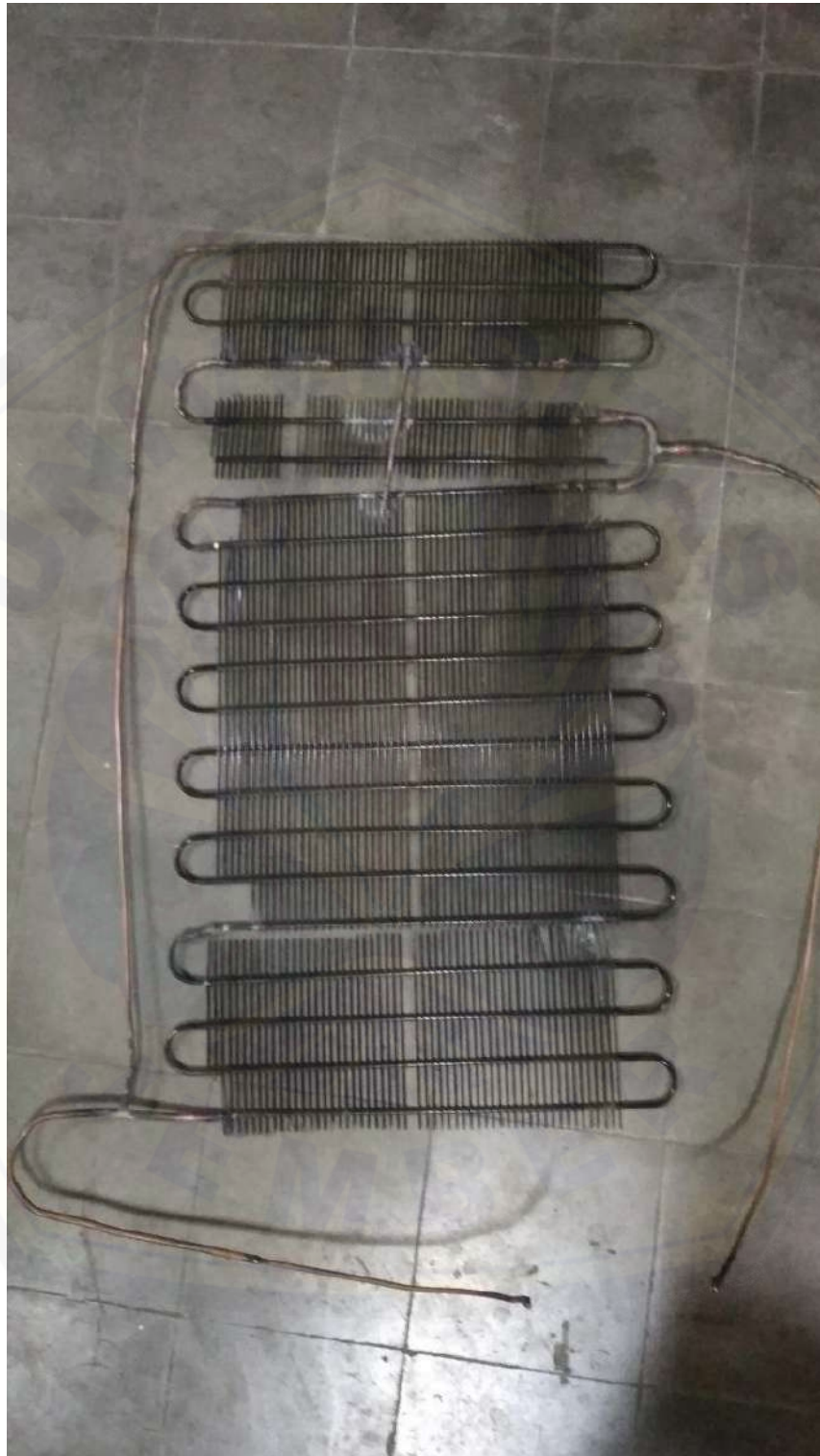
Gambar H.4 Separation Condenser Tipe C
