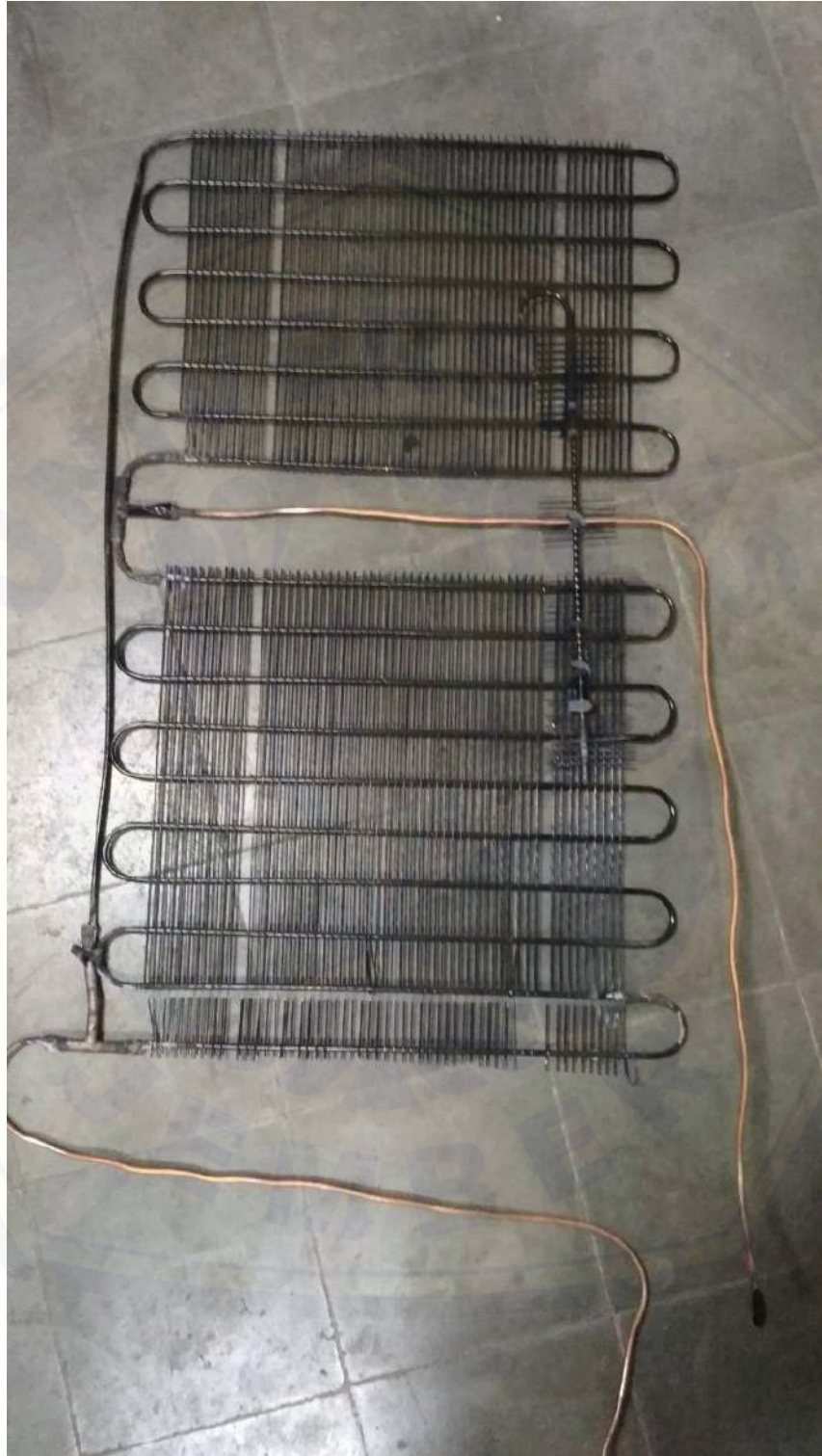
Gambar H.3 Separation Condenser Tipe B
