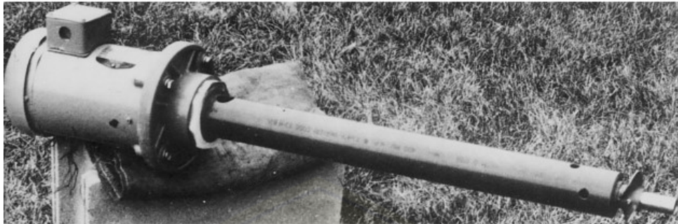
Gambar 2.3 Propeller aspirator pumps (Sumber: Boyd, 1998)
