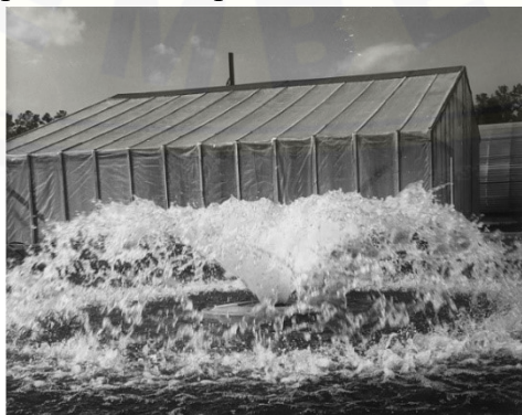
Gambar 2.1 vertical pumps aerator . (Sumber: Boyd, 1998)
