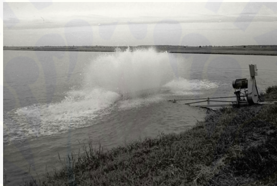
Gambar 2.2 Pumps sprayers aerator (Sumber: Boyd, 1998)
