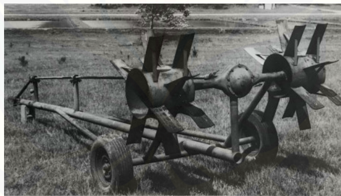
Gambar 2.6 Tractor powered aerator (Sumber: Boyd, 1998)
