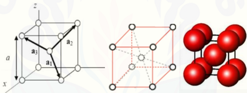
Gambar 2.2 Struktur kristal Body Centered Cubic (BCC) (Sumber: Jasprit, 2003)
