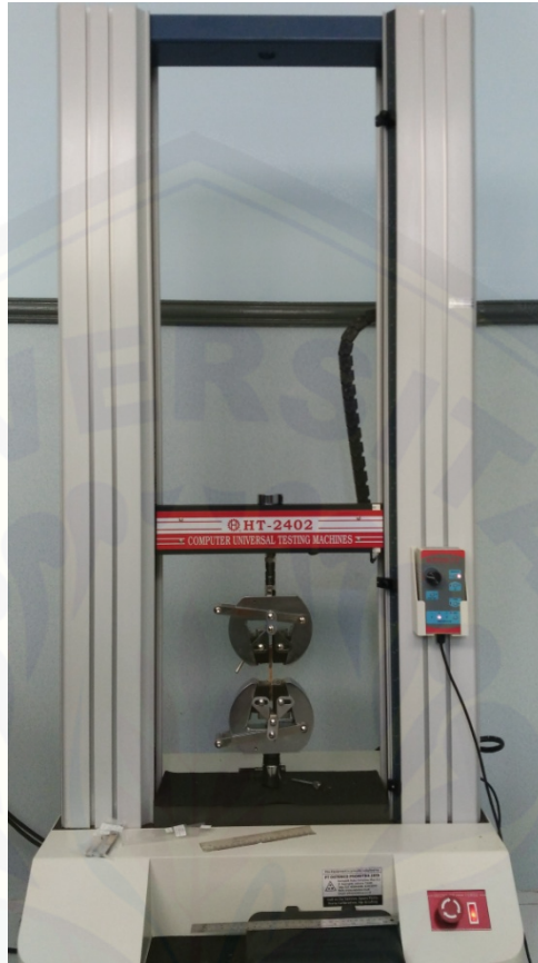
Gambar 3.5 Alat uji tarik Universal Testing Machine - UTM HT 2402-10kN
