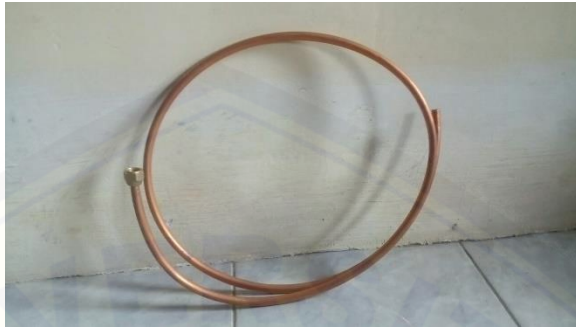
Gambar 3.3 Pipa Distribusi Uap
