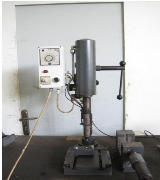
Gambar 3.1 Mesin *Injection molding*
