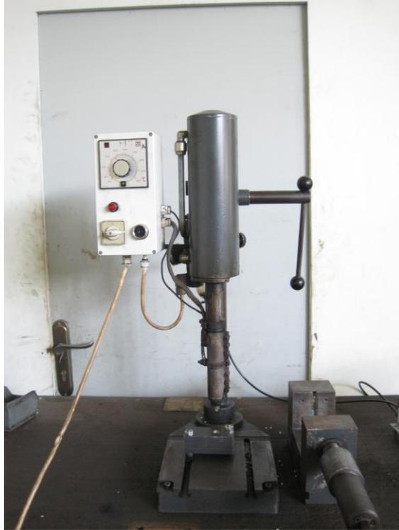
Gambar C.1 Mesin *Injection Moulding*
