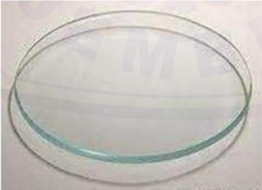
A clear, circular glass watch glass with a slightly raised rim, used for evaporating or drying samples.                                                                                                                                                                                         | Kaca Arloji                 |
