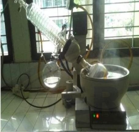
A rotary evaporator setup in a laboratory. It consists of a round-bottom flask containing a liquid, mounted on a motorized rotating platform. The flask is connected to a condenser coil that leads to a collection flask. The entire assembly is placed over a water bath on a magnetic stirrer. | Rotari Evaporator           |
