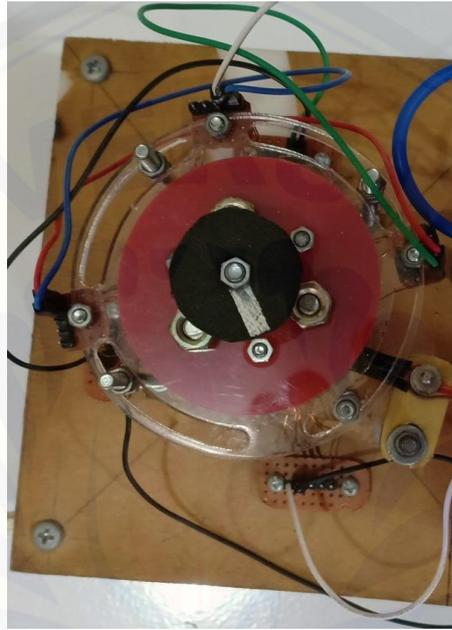
Gambar 3.6 Perancangan Motor *Brushless Direct Current Axial Flux* Tampak Atas
