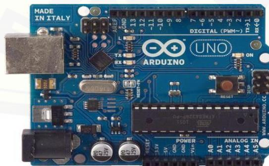
Gambar 2.3 *Board* Arduino Uno
