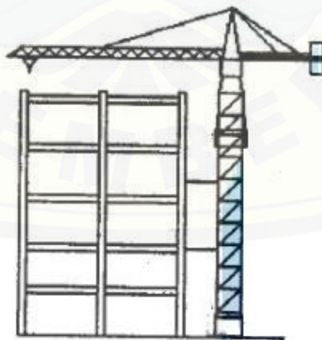
Gambar 2.3. Tied-in tower crane
