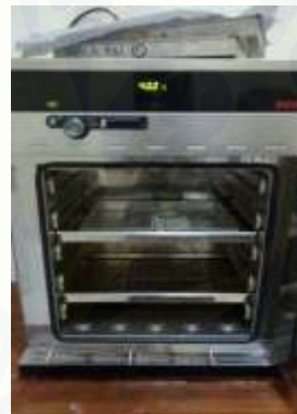
Hollow microspheres dioven selama 24 jam
