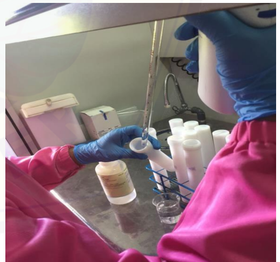
Gambar 12. Penambahan 5 mL Asam Nitrat Ultrapure ( \text{HNO}_3 ) 60%
