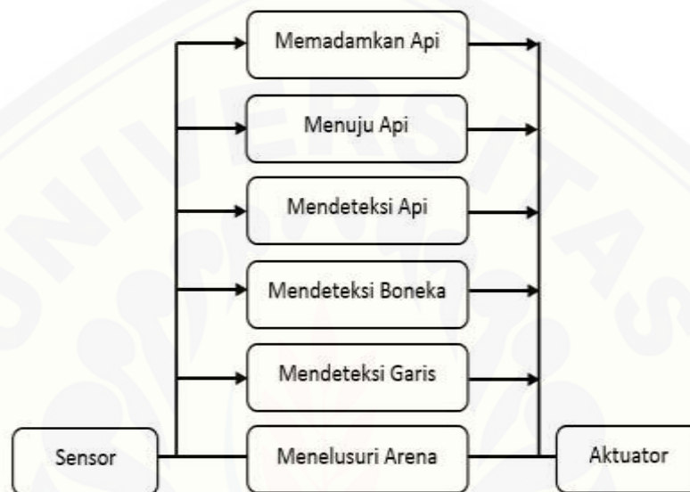
Gambar 3.11 Algoritma behaviour based control robot KRPAl berkaki
