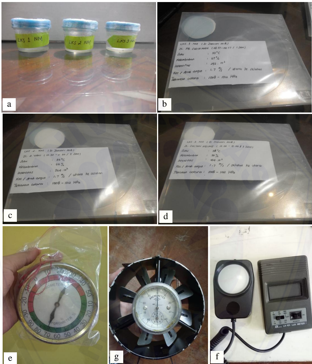
Gambar 1. a. Sampel larutan KI penjerap karbon monoksida (CO) tiga jalan protokol; b. Sampel filter timbal (Pb) Jalan PB Sudirman; c. Sampel filter timbal (Pb) Jalan Ahmad yani; d. Sampel Filter timbal (Pb) Jalan Sultan Agung; e. Termohigrometer; f. Anemometer; g. Luxmeter.
