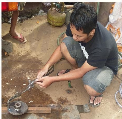
Gambar C.20 Proses brander cam
