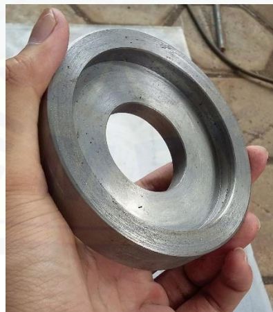
Gambar C.11 Dudukan noozle (Aluminium)
