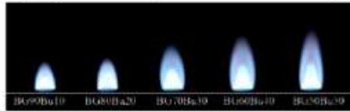
Figure 6 Changes in inner and outer fire cone height from combustion of biogas mixture with butane 10% -50%
