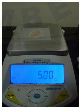
Gambar 3.15 Penimbangan powder bioactive glass (Sumber: Koleksi Pribadi)
