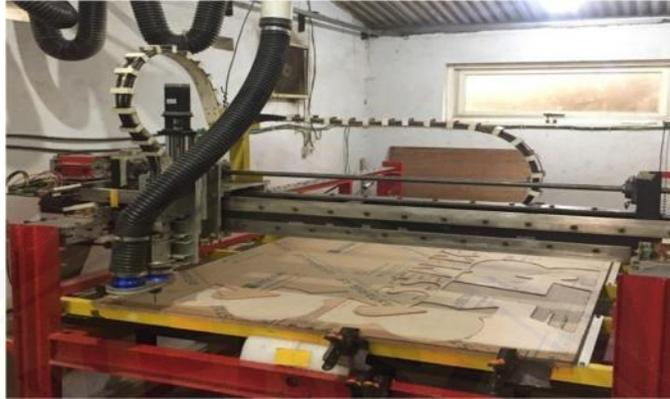
Gambar 2.4 Mesin CNC Milling DIY (Sumber: CNC jember 5, 2017)
