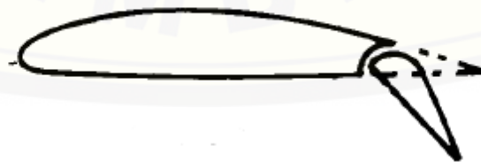
Gambar 2.8 Penampang single slotted flap (Raymer, 1992)
