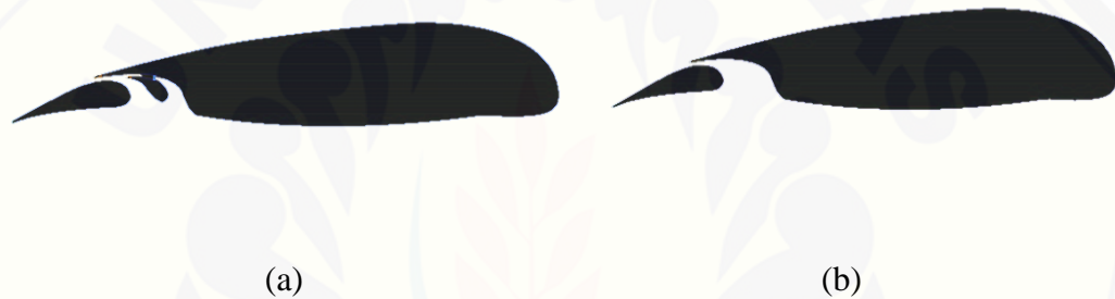
(a) Desain airfoil double slotted flap ; (b) Desain airfoil single slotted flap
