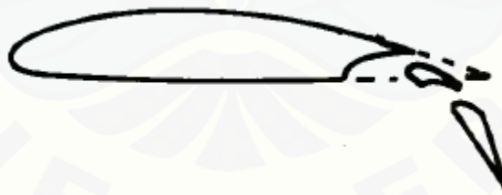
Gambar 2.10 Double slotted flap (Raymer, 1992)
