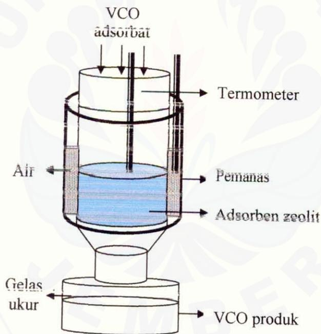
Gambar 2.12 Kolom *Fluid Fixed Bed*
