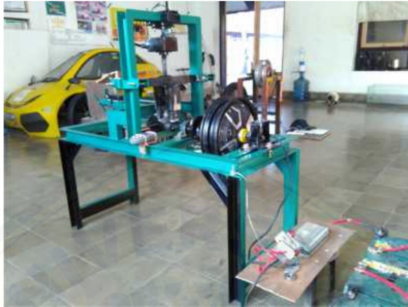
Alat uji rolling resistance bantalan
