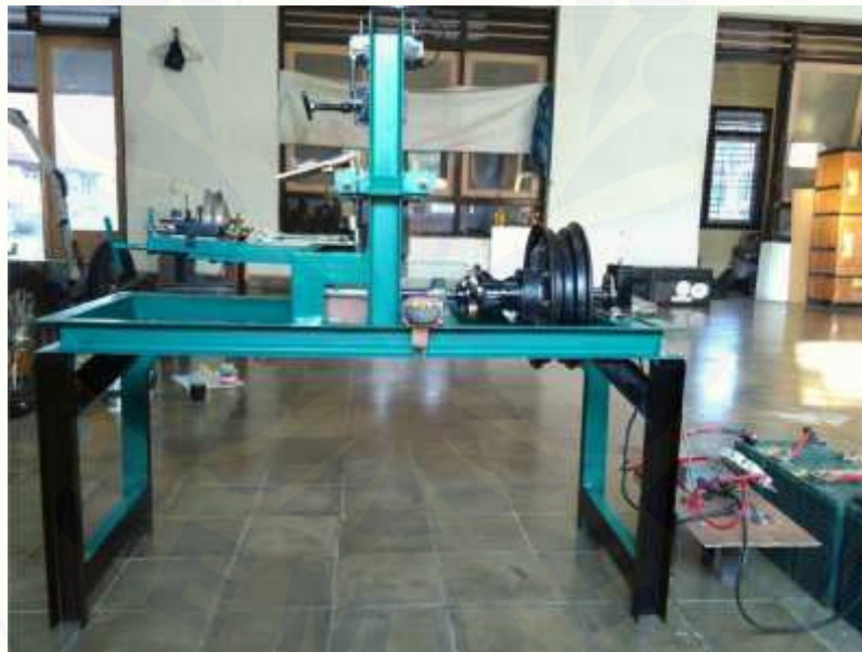
Alat uji rolling resistance bantalan
