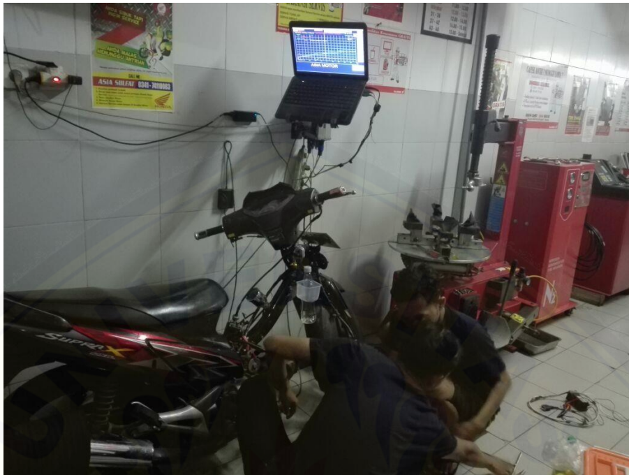
Lampiran D.1 Gambar pengujian dynotest
