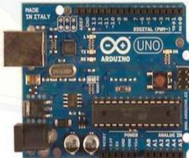
Gambar 2.1 Board *Arduino Uno*
