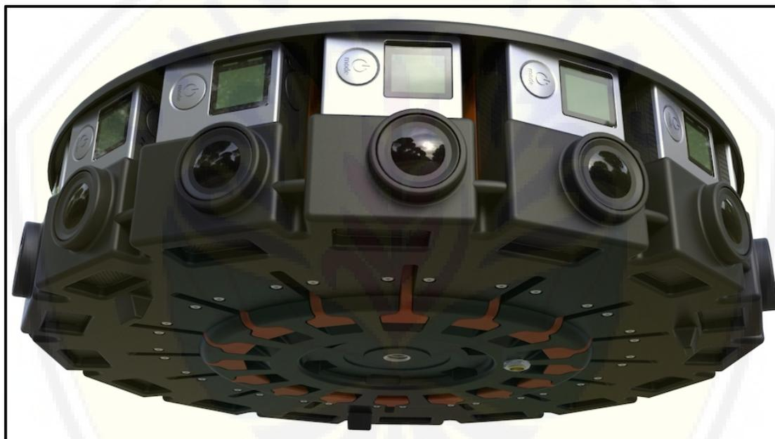
**Gambar 4.** Array: kamera 360 buatan Google (sumber: [https://cdn.vox-cdn.com/thumbor/Ot-QfgeWpWv6k-4gfa0makxCI8=/1020x0/cdn.vox-cdn.com/uploads/chorus\\_asset/file/3732294/gopro-google-camera-array-rig-0098.0.jpg](https://cdn.vox-cdn.com/thumbor/Ot-QfgeWpWv6k-4gfa0makxCI8=/1020x0/cdn.vox-cdn.com/uploads/chorus_asset/file/3732294/gopro-google-camera-array-rig-0098.0.jpg), diunduh 17 November 2017, 10.35 wib).
