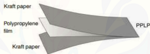
Gambar 2.4 Susunan Isolasi Paper-Insulated Oil-Filled Cables
